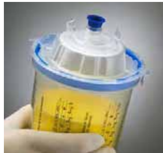
Insert the plug firmly into the lid tower if using a mechanical shaker or for storage until ready to use.
