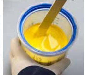
Mix paint by stirring (if not using a shaker) and clean liner flange/ring area of any paint before attaching to lid.
