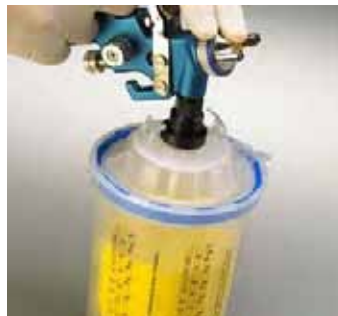
Mount the adapter flush to the lid tower base by pressing down firmly on the spray gun.
