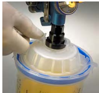
"Snap" the adapter locks over the adapter base to secure the lid to the gun adapter.
