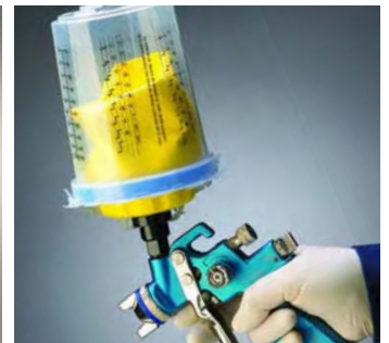
Connect air line to gun and purge air from the liner, adjust spray pattern and you're ready to spray.
